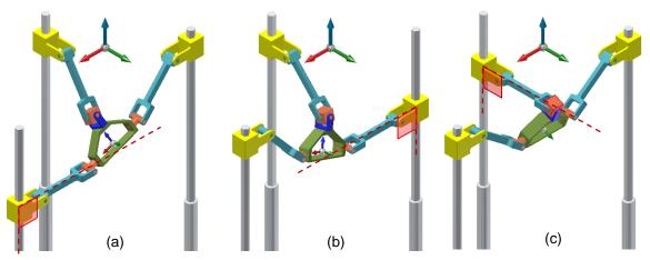
Figure 2. PRoM-120 configurations at the IKS or the input transmission singularity: (a) link  $B_1C_1$ , (b) link  $B_2C_2$ , and (c) link  $B_3C_3$  were perpendicular to the first, second, and third prismatic joint, respectively.
