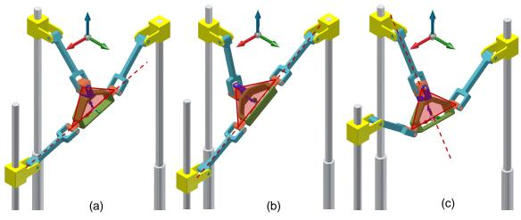
Figure 3. PRoM-120 configurations at the DKS or the output transmission singularity: (a) link  $B_1C_1$ , (b) both link  $B_1C_1$  and  $B_2C_2$ , and (c) link  $B_3C_3$  were in the plane to the platform plane, respectively.
