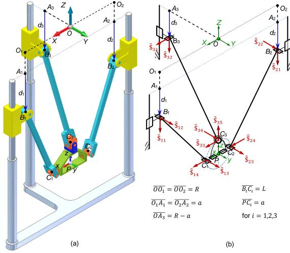
**Figure 1**. The geometrical architecture of PRoM-120 with 2-<u>PRU/PRS</u> kinematic chain: (a) simplified CAD model and (b) its kinematic diagram with the unit screw on each joint.
