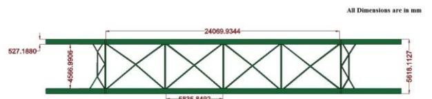
Figure 4: Top drawing of Truss Bridge
