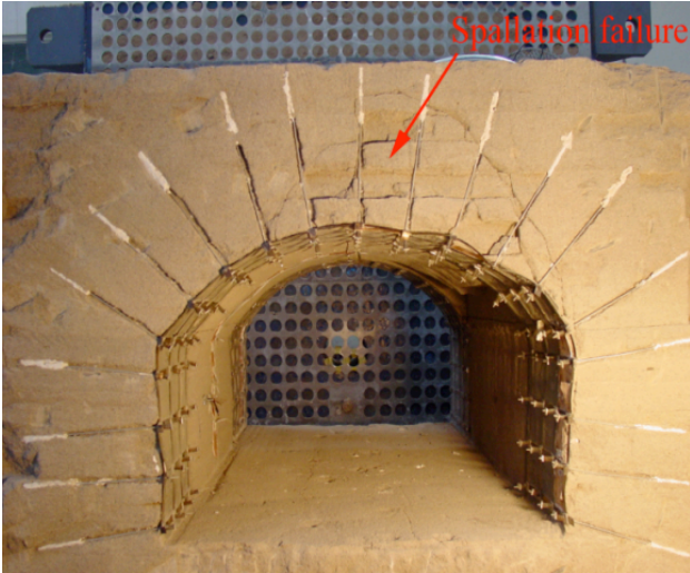
Fig. 5. Failure modes of the model tunnel reinforced by part-grouted anchor bolts
