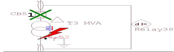
Figure 2. Fault Current at Secondary of Transformer (T3) & Circuit Breaker (CB5) Opening
