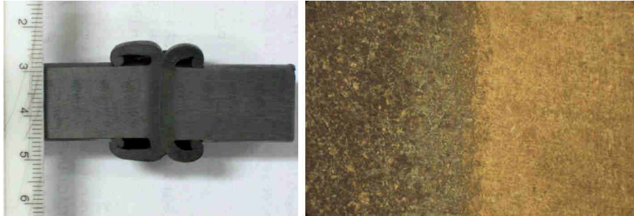
Figure 10. Sample no. 6: Macrostructure and shrunk area, 100x
