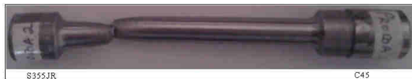
Figure 6. Sample no. 3 after the traction testing
