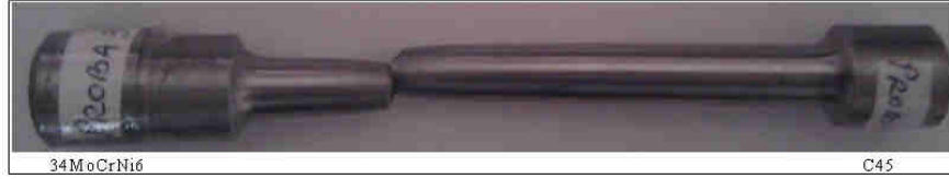
Figure 7. Sample no. 5 after the traction testing
