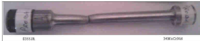
Figure 5. Sample no. 1 after the traction testing
