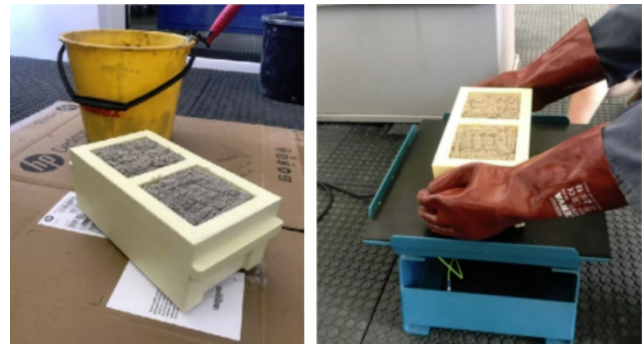
Figure 11. Filling and vibration
