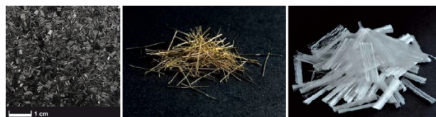
Figure 2. Carbon, steel and glass fibers [2]
