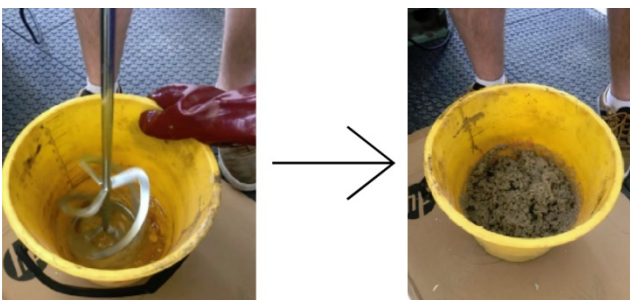
Figure 10. Mixing the matrix and the filler into the resulting mixture
