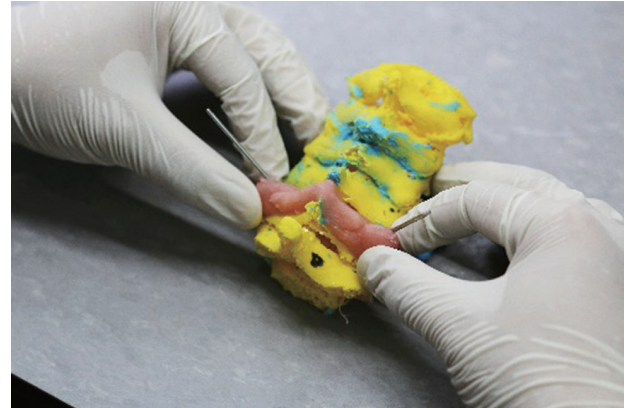
Fig. 5. Polymethylmethacrylate dental cement was molded on the posterior elements of the cervical spine models incorporating the Kirschner wires until it set into a firm molded drill guide.
