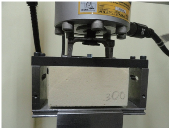
Fig. 3. Setup for pull-out strength study.
