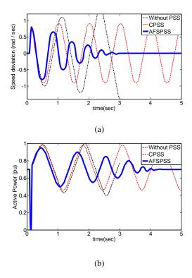
Fig. 4. Response for case 1: (a) rotor speed deviation; (b) active electrical power
