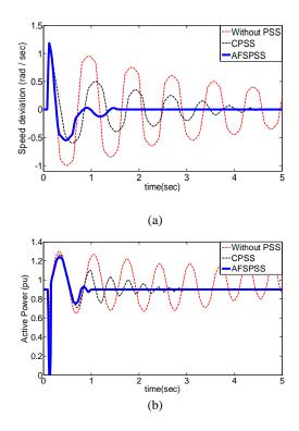
Fig. 5. Response for case 2: (a) rotor speed deviation; (b) active electrical power
