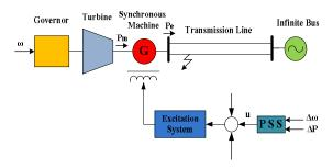
Fig. 2. Single machine infinite-bus power system
