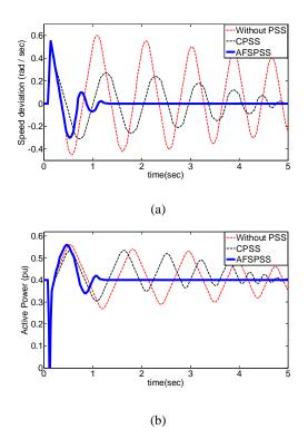
**Fig. 6.** Response for case 3: (a) rotor speed deviation; (b) active electrical power
