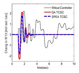
**Fig. 11.** Response of  $\Delta \omega_{13}$  for normal load condition
