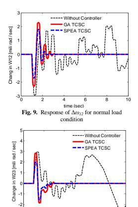
time(sec) **Fig. 10.** Response of  $\Delta \omega_{23}$  for normal load condition
