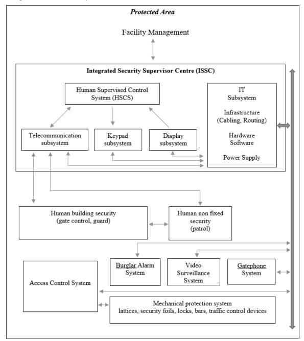
**Figure 1.** The model of the complex security system on a railway station.
