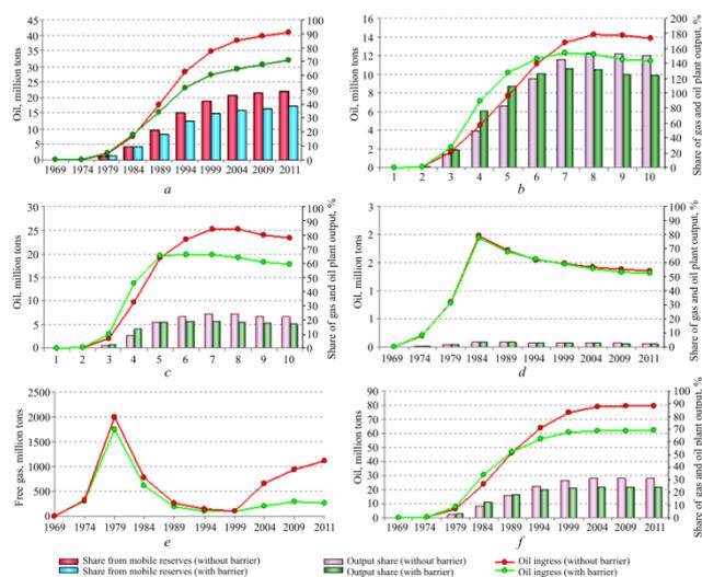
Figure 5. Dynamics of accumulated ingress volumes of oil into the gas cap and free gas into the oil zone: *a* – oil ingress into the gas cap, horizon AB<sub>1-2</sub>; *b* – oil ingress into the gas cap, horizon AB<sub>1-3</sub>; *c* – oil ingress into the gas cap, horizon AB<sub>2-3</sub>; *d* – oil ingress into the gas cap, horizon AB<sub>4-5</sub>; *e* – free gas volume below GOC, million m<sup>3</sup>; *f* – oil ingress into the gas cap, horizon AB<sub>1-5</sub>
