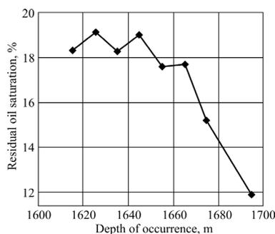
Figure 4. Dependence of residual oil saturation (determined by the sealed core sample) from true vertical depth for horizons AB<sub>1-5</sub> of Samotlor field (porosity is 24–28 %, true vertical depth of gas-oil contact – 1611 m)
