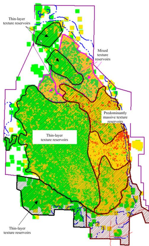
Figure 3. Schematic borders of various textures in horizon  $AB_1^{1-2}$
