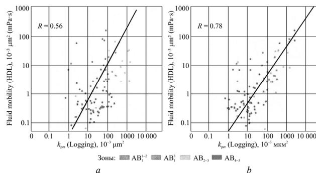
Figure 2. Comparison of fluid mobility by logging data and fluid mobility by HDL data for the old (a) and new (b) model
