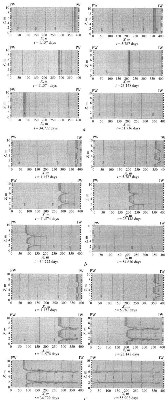
Figure 1. Pressure fields dynamics (isolines) and water saturation (color) for a homogeneous horizon with clay interlayers in the course of development by vertical wells: *a* –  $d = 0.0$ ; *b* –  $d = 20.0$ ; *c* –  $d = 10.0$ .  $Z$ , m – depth;  $X$ , m – width;  $t$  – time after well startup; PW – production well, IW – injection well
