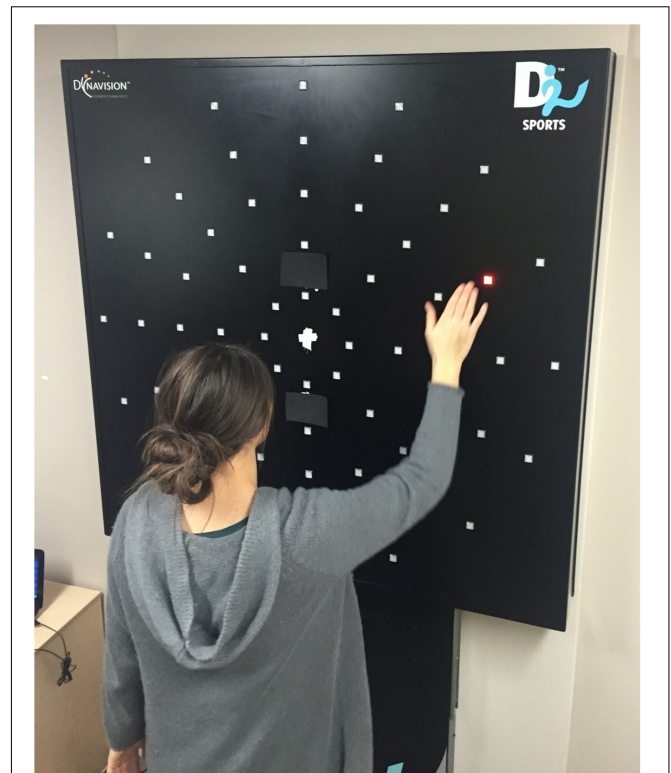
FIGURE 1 | A participant completing the DynaVision reaction time task. The participant fixated on the white cross in the center for the duration of the 60-s session. A single button would light up until the participant hit it. Reaction time for each button press was recorded. Both written and informed consent was obtained from participant for the publication of this image.
