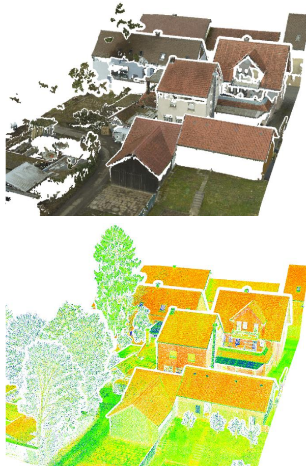
Figure 5. Comparison of photogrammetric (top: RGB colored) and LiDAR point cloud (bottom: colored by reflectance – blue = low, red = high).
