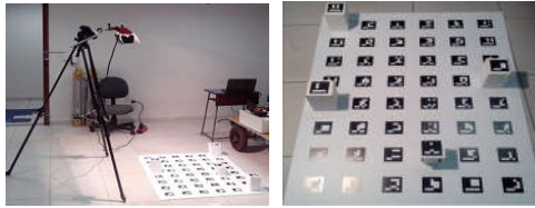
Figure 2. (a) Calibration set up, with the camera static and a targets plate; (b) example of one acquired image.
