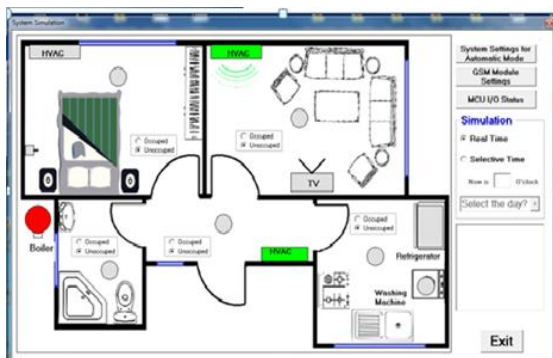
Figure 23: The Status ON for the HVAC in the corridor.
