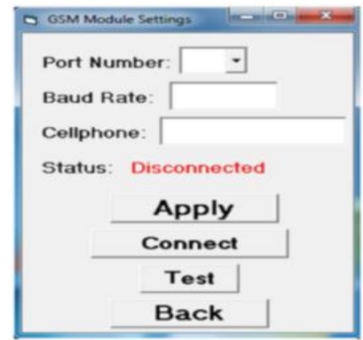
Figure.10: GSM module setting interface.
