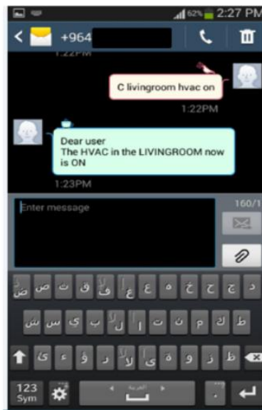
Figure 18: The sent and received SMS of test 1.
