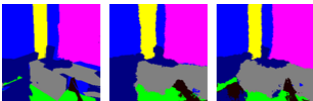
Figure 5. Improvement of the labeling at the boundaries using depth on example of class column (yellow). The images represent: ground truth (left), RGB based label prediction (middle), R_dG_dB_d based label prediction
