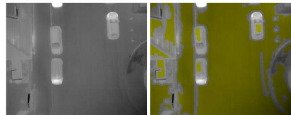
Figure 2: Uniform region detection: left is the raw TIR image, right is the TIR image with detected uniform regions (shown in yellow)
