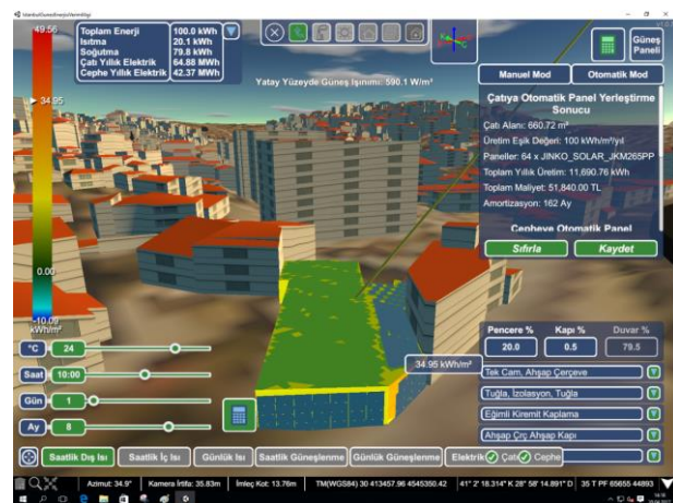
Figure 18. Solar estimation for the selected building rooftop and façade (potential solar panel).
