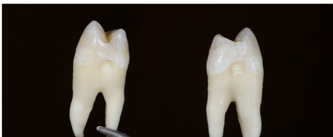
Fig. 1. Round artificial cavities (3×1 mm) on tooth proximal surfaces.
