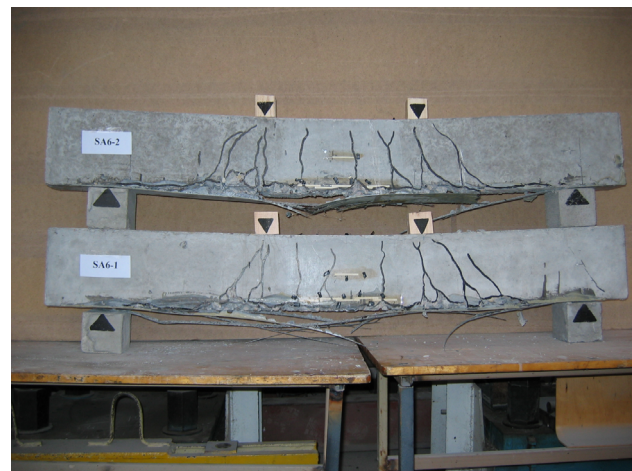
Fig 10. Crack pattern of SA6 series beams
