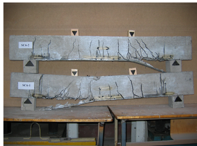
Fig 11. Crack pattern of SC6 series beams
