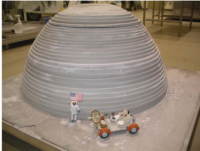
Fig. 3. Scaled prototype of lunar dome structure printed with Contour Crafting (CC). Credits Behrokh Khoshnevis, University of Southern California, USA.
