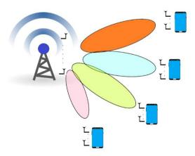
Fig. 1. Illustration of Multi-user MIMO Model
