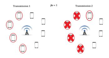
Fig. 3. Illustration of the proposed user selection concept
