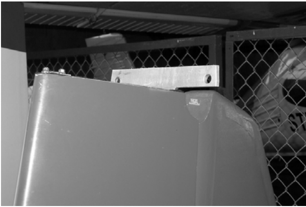
Fig 13. Beam joint on vertical stabilizer
