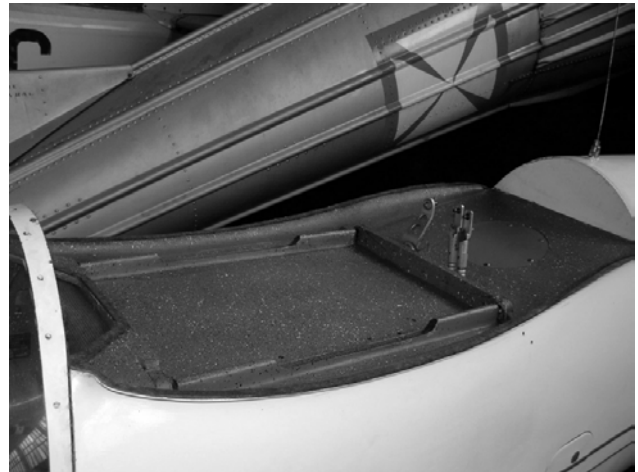
Fig 16. Clasps for attaching pins in fuselage centre section
