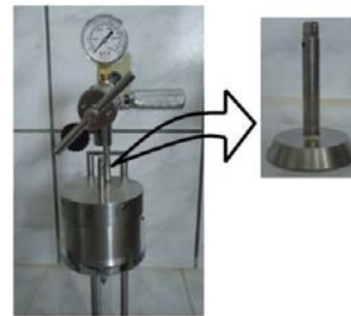
Figure 1: Differential sticking tester by Fann and the radius plate.
