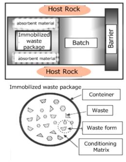
Fig. 5. Components of the storage system.
