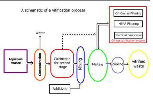
Fig.4. A schematic of vitification, using borosilicate glass.
