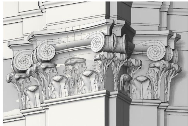
Figure 8. Mathematical model of the angular composite capital.
