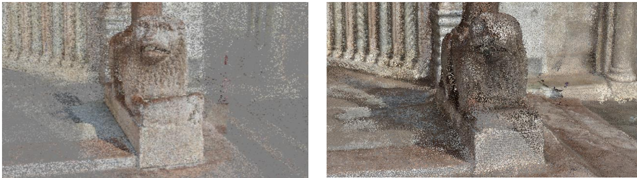
Figure 2: An example of the sparse (left) and dense (right) point cloud produced by jointly processing UAV and terrestrial images featuring different scales, viewpoints, etc. The final dense cloud is noisy and with visible misalignments, due to inaccurate orientation results.
