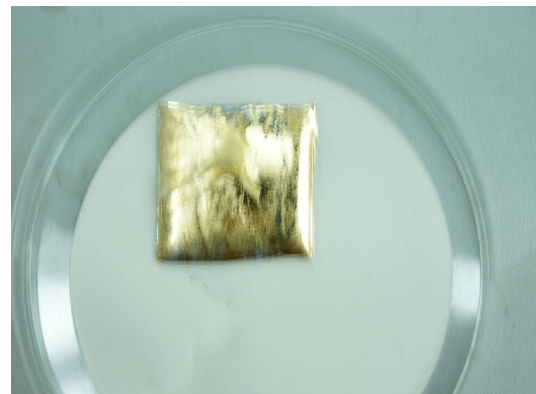
Fig. 2. The substratum Au electrode on PDMS film.
