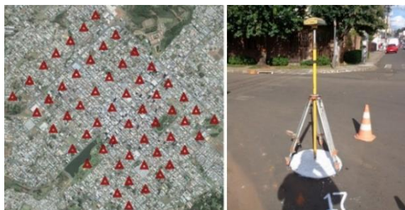
Figure 4: (a) Layout of control points. (b) Circular design signalized at the ground. (Ercolin Filho et al., 2017)
