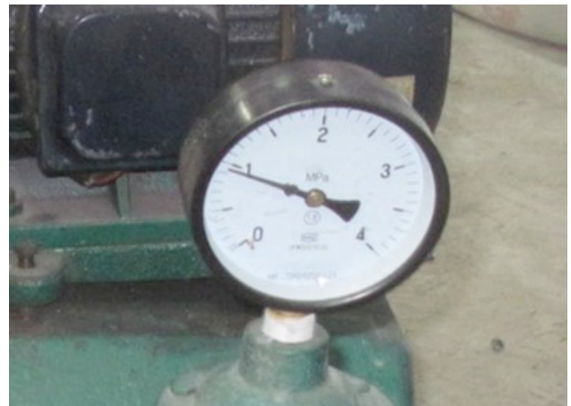
Fig. 15. Final grouting pressure under dynamic water pressure and confining pressure
