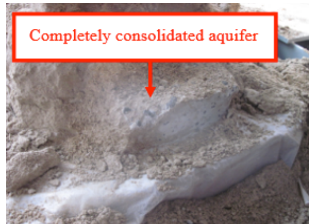
Fig. 9. Grouting effect of aquifer under no dynamic water pressure or confining pressure
