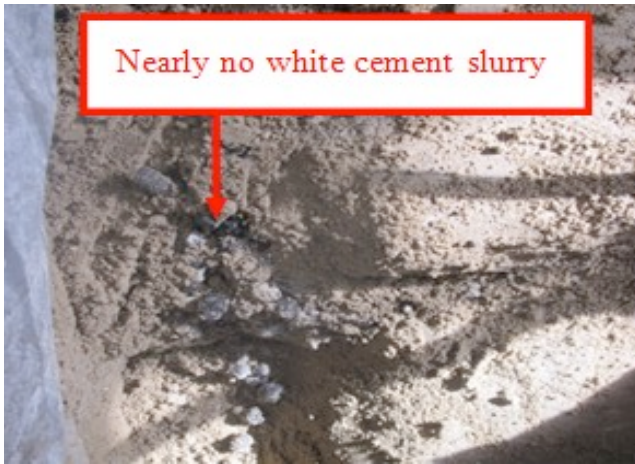
Fig. 12. Grouting effect of aquifer under dynamic water pressure and confining pressure
