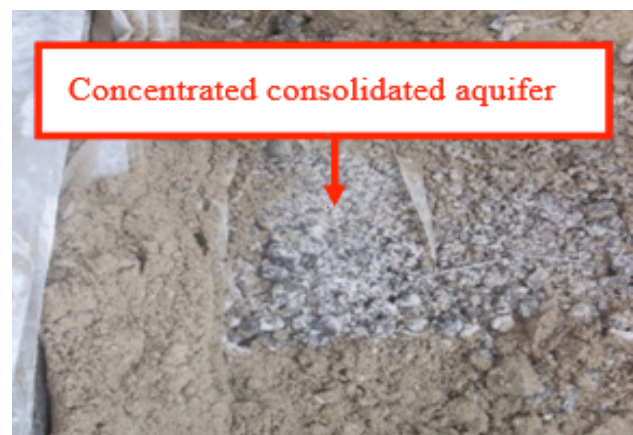
Fig. 11. Grouting effect of aquifer under confining pressure only
