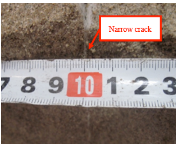
Fig. 8. Grouting effect of cracks under triaxial pressure only
