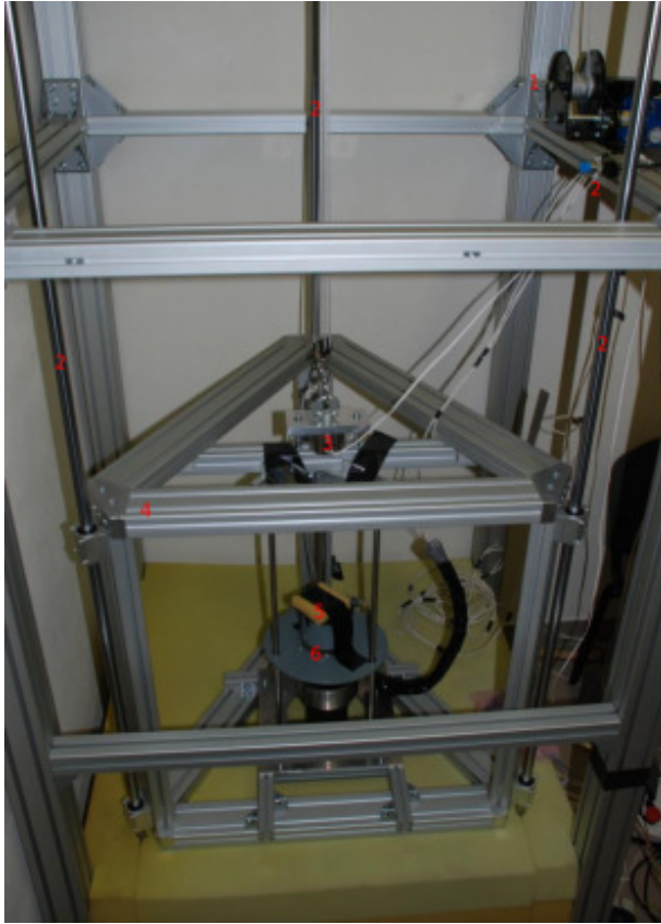
FIGURE 1. Drop tower setup (1 - motorized drop-weight lift, 2 - trigger inductive sensor, 3 - guide rods, 4 - electromagnetic release member, 5 - drop-weight guide frame, 6 - accelerometer, 7 - drop-weight).
