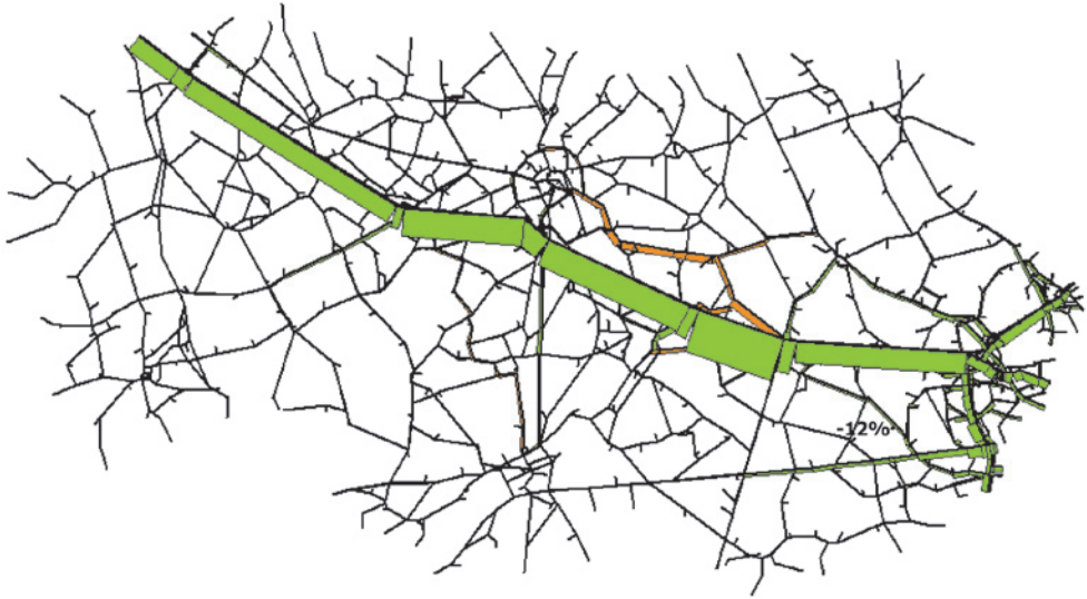
a) Change in traffic flows for a cordon toll of 1 euro around Brussels, a corridor toll on E40 (5 euro) and a tolling point (1 euro) near Aalst. Light colour (green) is decrease, dark colour (red) is increase in traffic flow
