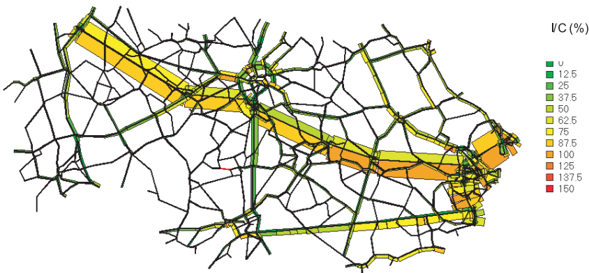
Fig. 2. Current situation, bandwidth = load in morning peak, colour = I/C ratio (see the text for further information)
