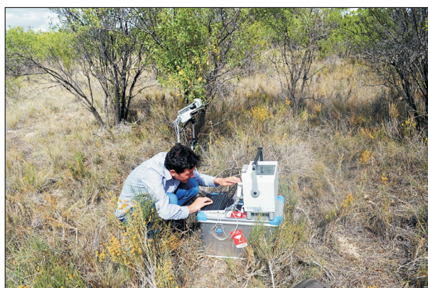
Fig. 1. Gas exchange measurements of the Arabian almond tree in the field of Konya Karapınar.
