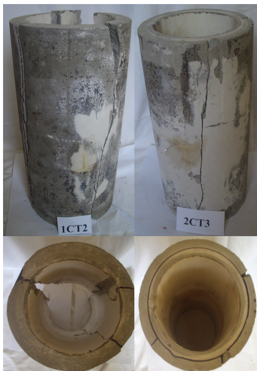
Fig 14. Single- and double-layered H-CT tested specimens
