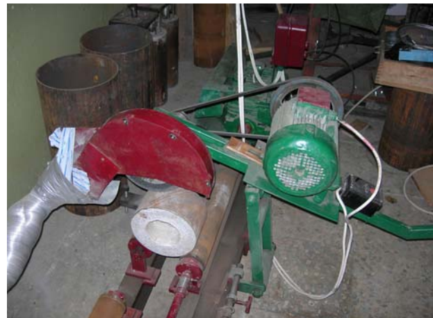
Fig 2. Cutting machine used for preparing the specimens
