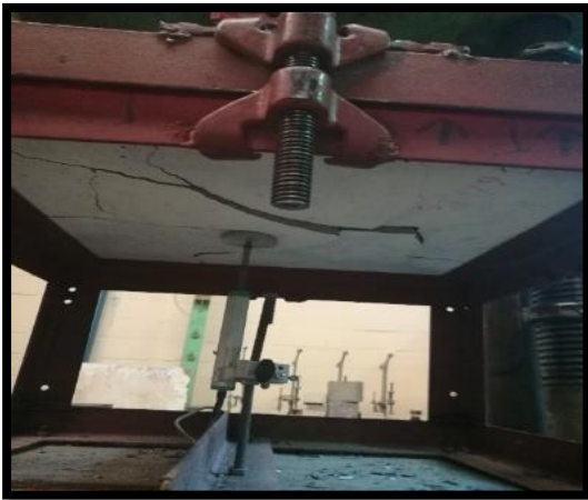
Plate 4: Bottom failure of SCMs fibre reinforced plate.
