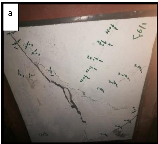
Plate 6: Crack pattern of 3D textile fibres 6mm, a) One layer. b) Two layers.
