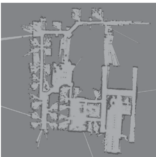
(e) The map built using tinySLAM
