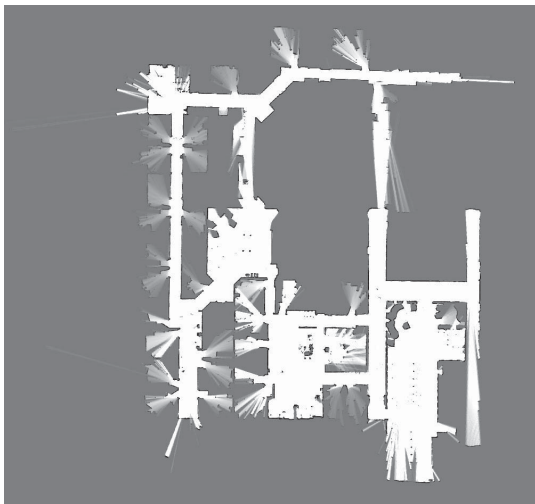
(c) The map built using Cartographer
