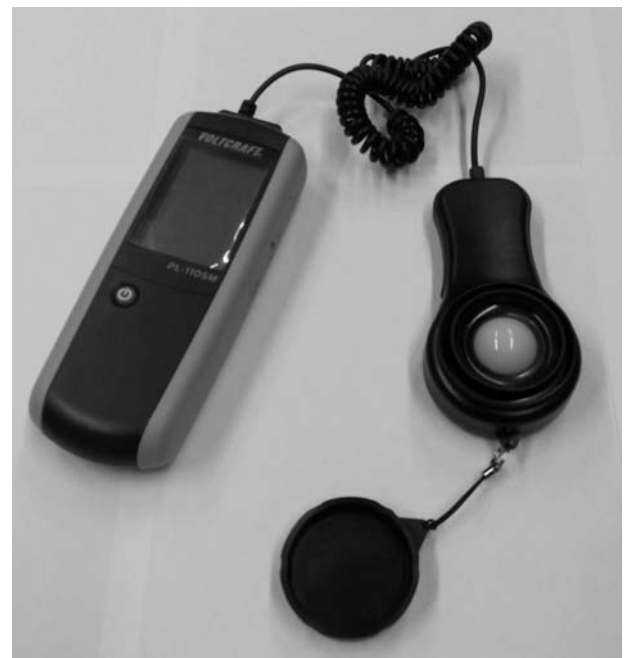
Fig. 19. Voltcraft PL-110SM solar radiation measurement instrument
