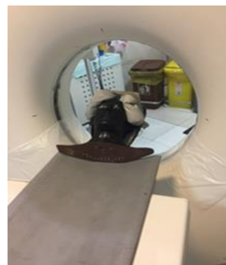
Figure 4. Locating the phantom in the gantry fixed in head CT protocol position and locating the dosimeters on the phantom as one TLD in an empty capsule on each eye and each thyroid lobe, followed by fixing by tape
