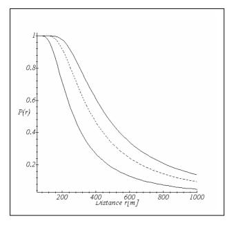
**Fig 4.** Dependence of probability of the detection of the enemy P(r) from the distance to it. Upper curve corresponds to time of observation 15 *s*, dotted – 10 *s*, lower – 5 *s*
