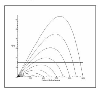
**Fig 6.** AK 74 bullet trajectories when shooting from 100 m to 1000 m distance. The top line corresponds to the shadow height of the attacking soldier -1.5 m - and the bottom line to that of the defending soldier -0.3 m
