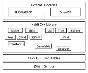
Fig. 1. Structure of the Kaldi ASR tool.
