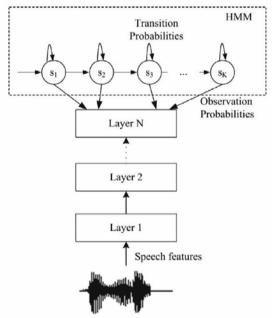
Fig. 2. Architecture of the DNN-HMM hybrid system.
