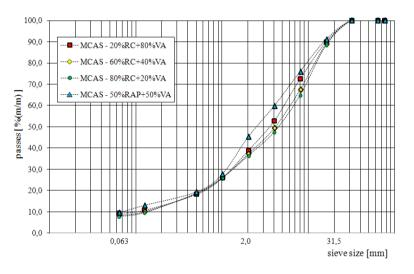
Fig. 1. Particle size distribution of analysed MCAS mixes
