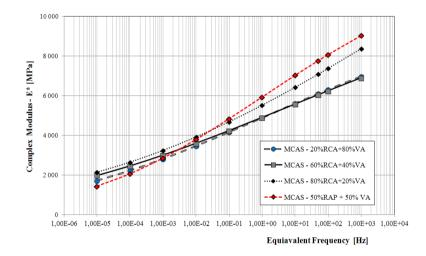
Fig. 2. Master curves for the analysed MCAS mixes (T<sub>ref</sub>=25°C)
