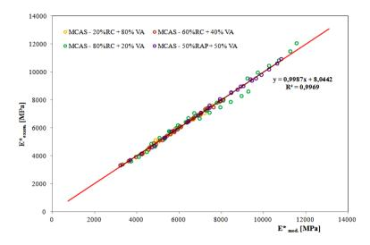
Fig. 3. Evaluation of the goodness of fit of complex modulus  $E^*_{exam}$  to  $E^*_{mod}$ .
