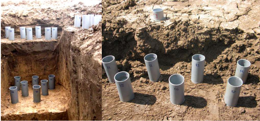
Fig. 3. Elements of tube method application for measuring of water permeability characteristics of various soil layers (45°32'10.6"N 34°11'38.0"E; 05.08.2016, Klepininsky settlement territory, Krasnogvardeysky district).
