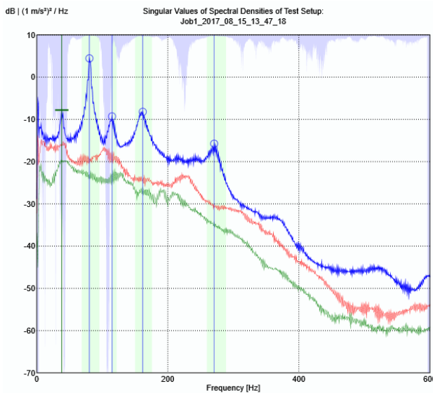
Fig. 7 Natural frequencies of the 0° laminated plates computed with ARTEMIS OMA
