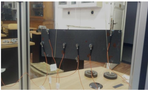
Fig. 6 Instrumentation of the 0° laminated plate for OMA
