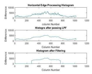
Fig.8. Vehicle plate extraction using Sobel edge detector (Horizontal Processing)
