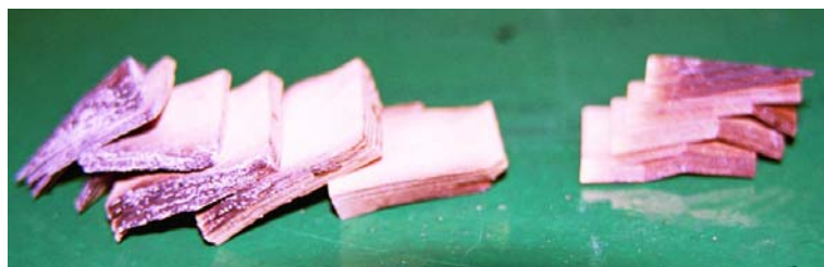
Fig 14. Damage character for impregnated samples after compressive strength tests above 200 °C:
