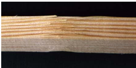
Fig 13. Long-fibre fractures of natural samples after static bending tests: a) at 20 °C; b) at 200 °C
