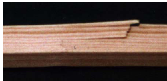
Fig 13. Long-fibre fractures of natural samples after static bending tests: a) at 20 °C; b) at 200 °C
