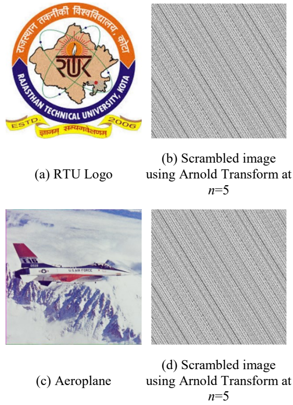
Fig.7. Scrambled image of RTU Symbol and Aero plane using Arnold Transform at n=5 iteration
