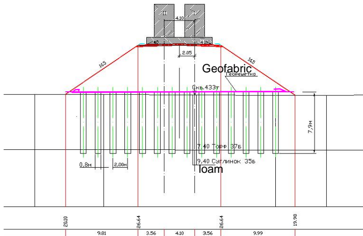
Fig. 2. The cross section of embankment (height 7 m) on peat foundation with a sand column.
