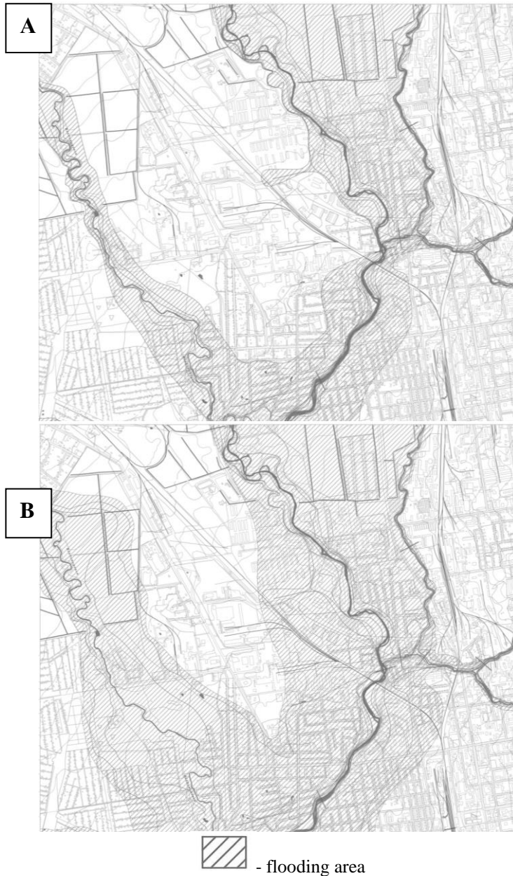
Fig. 1. The planning restrictions to the settlement general plan layout example (the flooding danger in Yuzhno-Sakhalinsk, occurrence of A - 1% and B - 0,1%).
